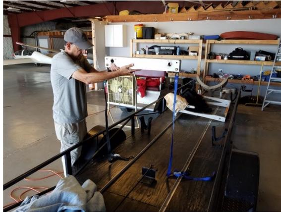
Place the fuselage cradle at the rear of the trailer. Elevate the trailer tongue. Place the wooden ramp at the end of the trailer. Roll, pull fuselage onto the cradle. Move the fuselage forward until the cradle engages the cradle latch. Make sure canopy is closed and latched. Install access cover on top of fuselage.
